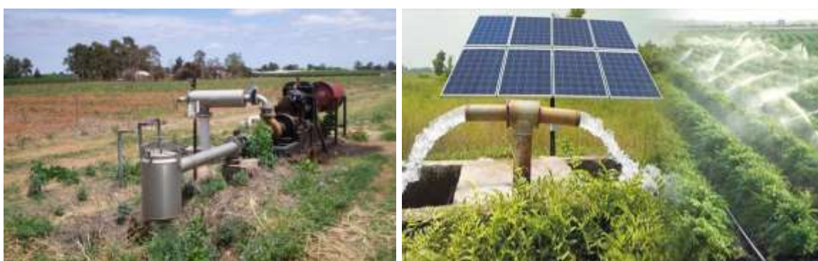
Figure 3: Fuel Powered and Solar Powered water pumps used in two irrigation systems
